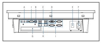
A: Line in/Line out/Mic in B: PS2 Mouse&Keyboard C: USB 2.0 x 4 D: VGA Port E: Power Switch
